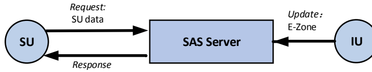
Figure 3.1: The architecture of E-Zone-based SAS
